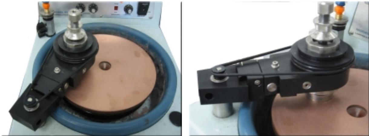
**Figure 4:** The Model 92003 Non-Contact Polishing Arm is shown as mounted to the Model 920. The holder is attached to the post of the Model 920 using a clamping screw arrangement. Horizontal and vertical alignment is done using adjustment screws with the sample mounting block attached. Samples are removed from the holder using a threaded knob arrangement as with the lapping and polishing fixtures.
