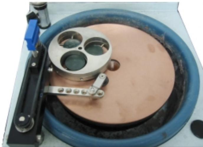
**Figure 5:** Model 92005 Tri-Holder Specimen Mount shown used with the Model 92002 Workstation. Metallographic samples can be processed simultaneously using this holder and can be applied to grinding papers, polishing cloths, or lapping techniques.
