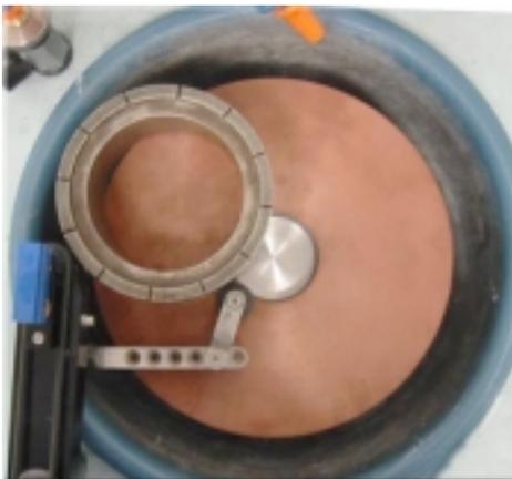
**Figure 9:** Image showing the Model 92002 Workstation with a diamond conditioning ring. The ring is used for removing material from the lapping plate surface to create a flat surface for lapping processes.
