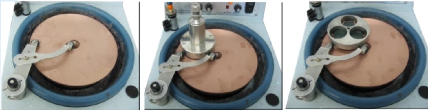
**Figure 8:** Various setups using the manual specimen yoke. At left is the yoke without any fixtures, while the center and far right images show the yoke with a Model 155 Lapping Fixture and the Model 92005, respectively.
