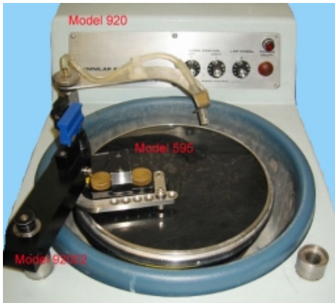
Figure 2: Figure 2 shows the basic arrangement for holding the Model 595 BiPod Polisher™ onto the Model 920.
