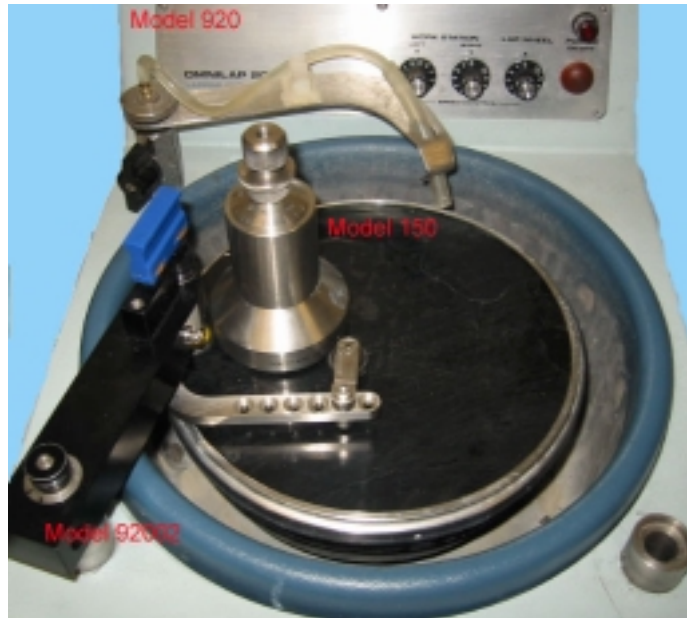
Figure 1: Figure 1 shows the basic arrangement for holding the Model 150 Lapping and Polishing Fixture.
