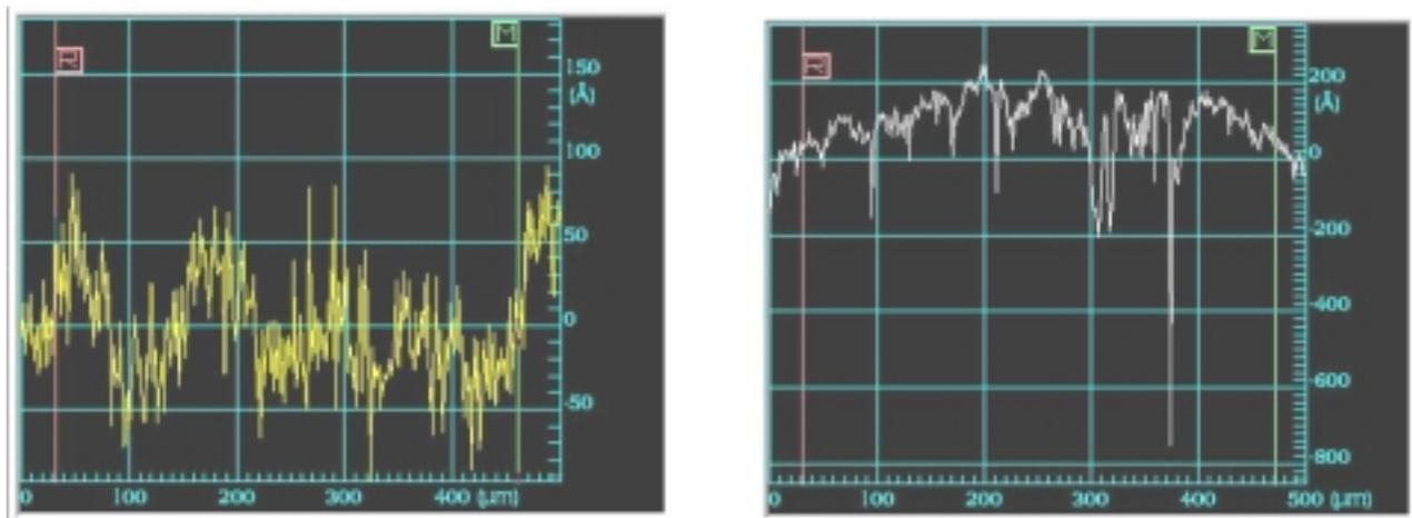
**Figure 7:** Surface profile scans of silicon wafer sample after polishing with 1  $\mu\text{m}$  diamond suspension on Nylon (left) and Rayon Fine (right). The Ra was given as 24Å for sample 16 at left and 57Å for sample 6 at right.
