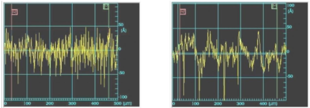
**Figure 2:** Surface profile scans of silicon wafer sample after polishing with 0.5µm (left) and 1 µm (right) diamond lapping films. The Ra was given as 15 and 17 Å, respectively.
