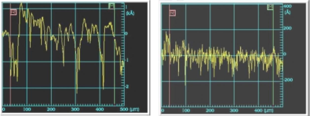
**Figure 6:** Surface profile scans of silicon wafer sample after polishing with 6  $\mu\text{m}$  diamond suspension on ChemoTex™ (left) and SanyPol™ (right). The Ra was given as 463Å for sample 10 at left and 40Å for sample 9 at right.
