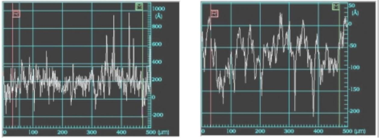
**Figure 8:** Surface profile scans of silicon wafer sample after polishing with 1  $\mu\text{m}$  aluminum oxide suspension on MultiTex™ (left) and Rayon Fine (right). The Ra was given as 94Å for sample 4 at left and 32Å for sample 5 at right.
