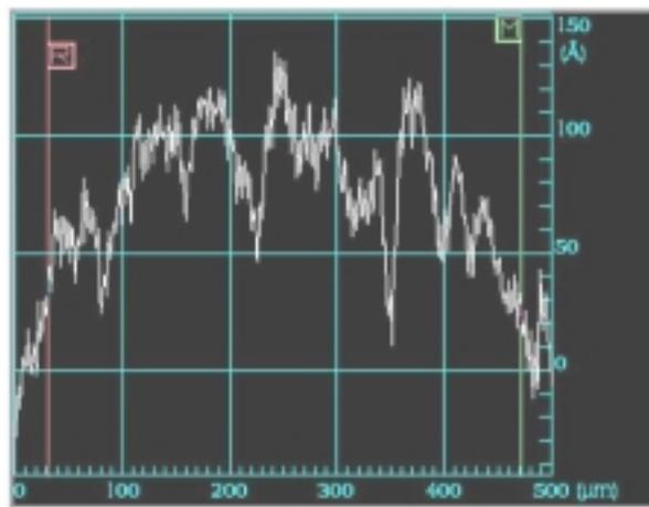
**Figure 9:** Surface profile scan of silicon wafer sample after polishing with 0.05  $\mu\text{m}$  colloidal silica suspension on MultiTex™. The Ra was given as 22Å for sample 3.
