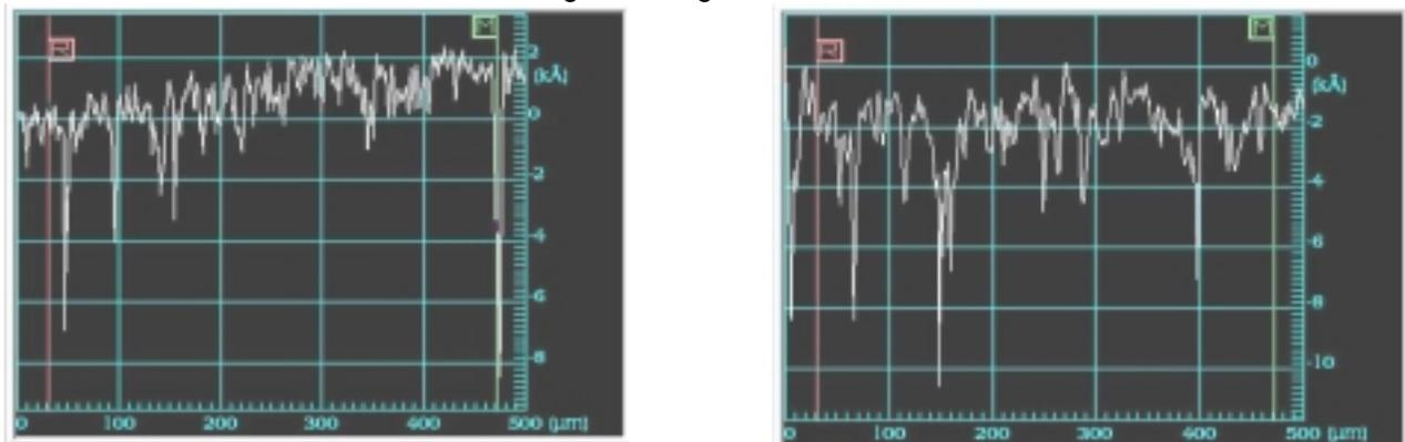
**Figure 4:** Surface profile scans of silicon wafer sample after lapping with diamond suspension on Cu composite plate using two different 15  $\mu m$  diamond suspensions. The Ra was given as 608Å for sample 11 at left and 879Å for sample 13 at right.
