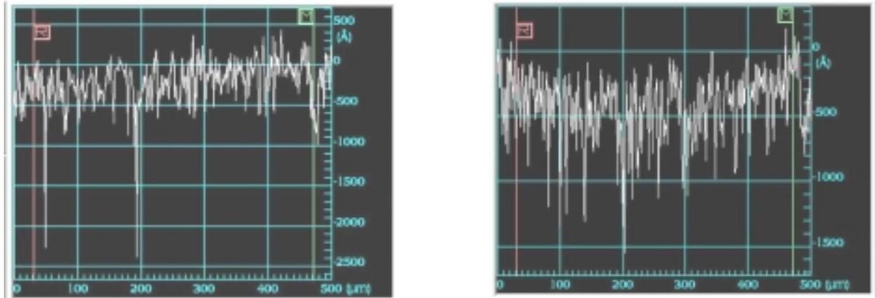
**Figure 5:** Surface profile scans of silicon wafer sample after lapping with diamond suspension on Cu composite plate using two different 3 μm diamond suspensions. The Ra was given as 185Å for sample 12 at left and 195Å for sample 14 at right.
