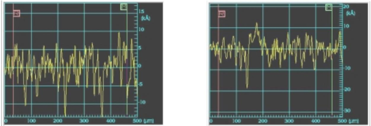
**Figure 3:** Surface profile scans of silicon wafer sample after lapping with aluminum oxide suspension on glass plate (left) and cast Fe plate (right). The Ra was given as 3140 and 3382 Å, respectively.
