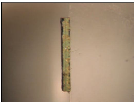
Figure 9: Cut specimen mounted up to pyrex stub edge
