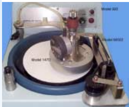
Figure 1: Image showing the Model 147D Lapping and Polishing Fixture mounted onto the Model 920 Lapping and Polishing Machine. The Model 147D is rotated and held in place using the Model 92022 Workstation. Oscillation of the fixture across the lapping plate surface is possible but was not used in this application.
