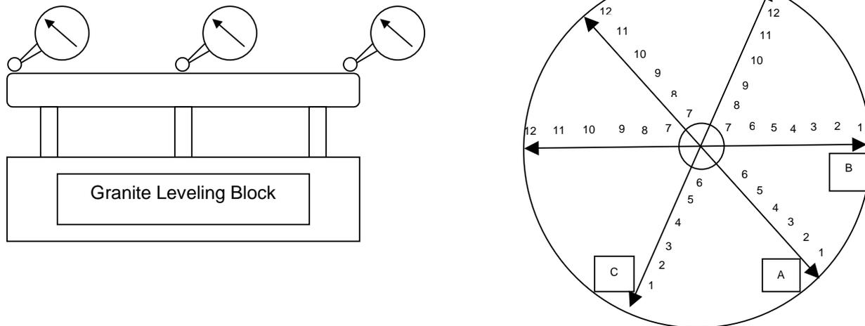
**Figure 1:** Schematic illustration of the technique used for measuring plate flatness. The plate is first made parallel on a granite leveling block using a dial gauge and three adjustment legs. After the plate is level, measurements are taken at various points on the surface of the lapping plate with the dial gauge. Each data point is then plotted to provide a surface plot illustrating the flatness of the plate after any given process.
