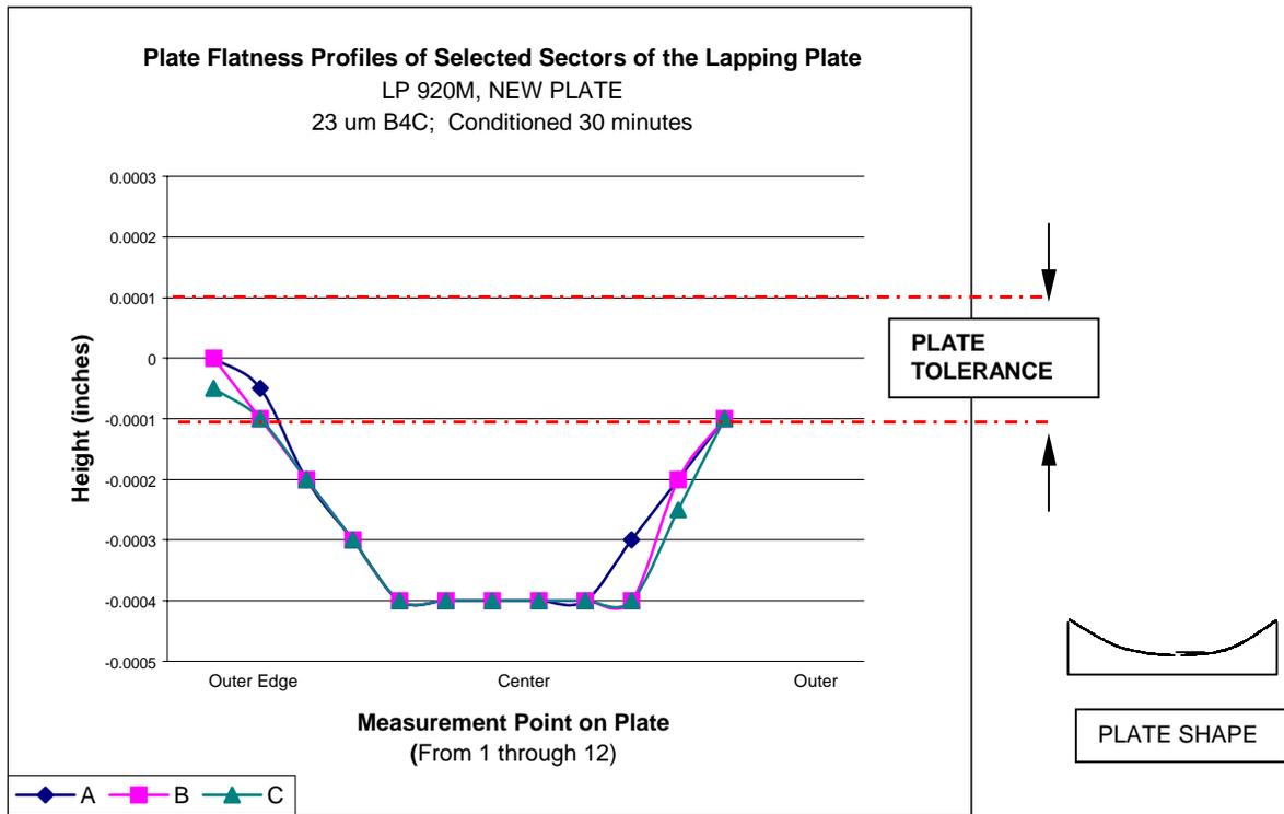
**Figure 4:** Plot of a new cast iron lapping plate following conditioning using the 'standard' conditioning ring method. As can be seen, the plate has flattened at the bottom, however no appreciable change in the plate shape can be observed. The plate still has a severe concave shape that will hinder proper specimen preparation.
