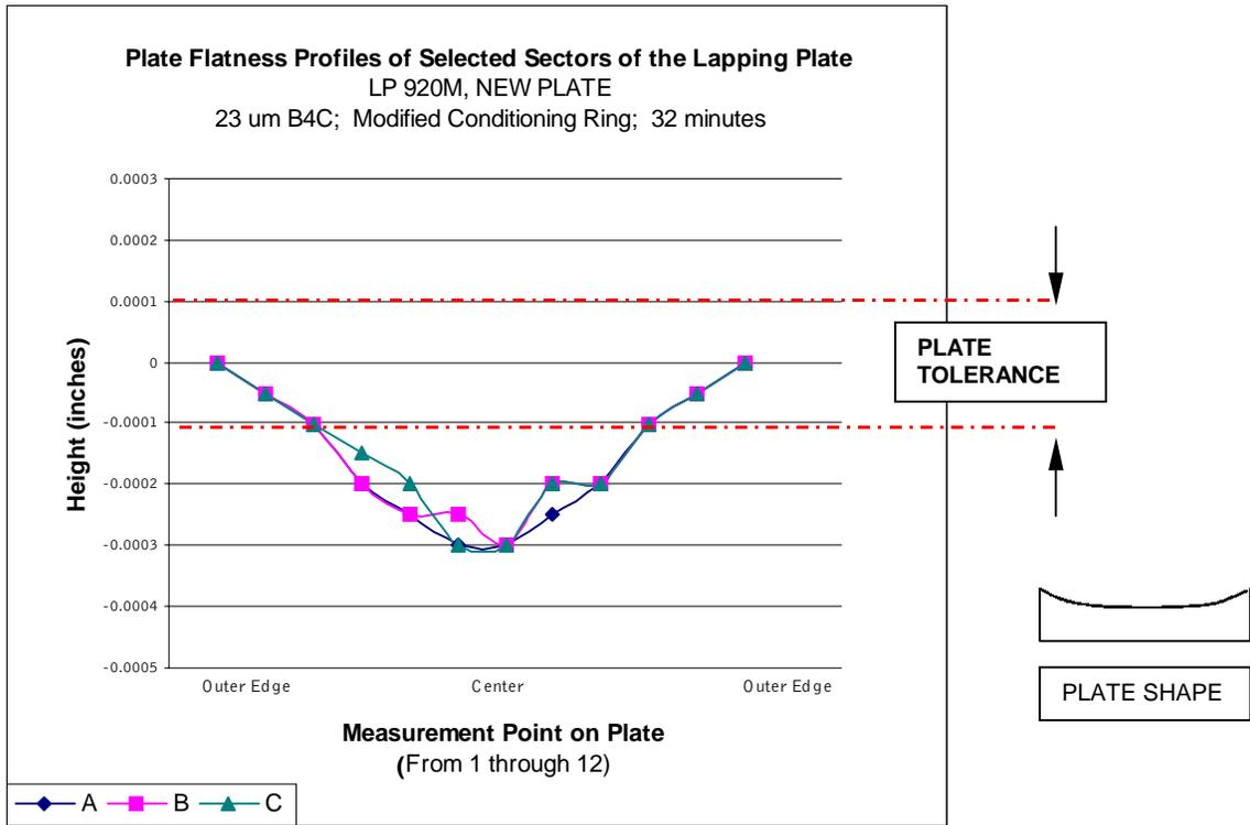
**Figure 5,6:** Plot of cast iron lapping plate following conditioning with the modified arrangement. As can be seen in Figure 5 (above) the lapping plate has become close to the tolerance limits specified in the manufacturing drawings of the plate, indicating conditioning using the modified arrangement is much more effective in producing flat plates. In Figure 6 (below) the plate has been conditioned to be within the specifications of the lapping plate.
