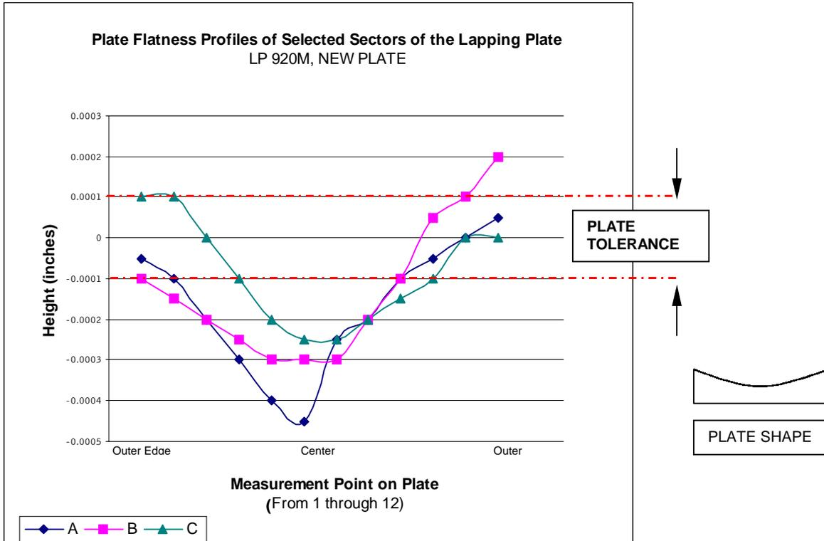
**Figure 3:** Plot of a new cast iron lapping plate prior to use. The plot shows three plotted series which represent the data series A, B, and C shown in Figure 1. From this plot you can see that the lapping plate is far from the tolerance specifications given for new lapping plates. The plate is dipped in the center, creating a concave plate shape.
