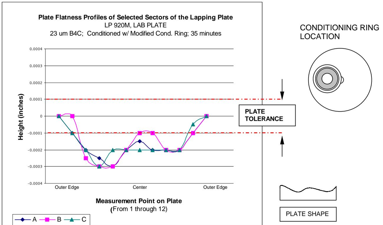
**Figure 7,8:** Plot of the plate surface following conditioning for 35 minutes. Figure 7 (above) shows the plate surface is beginning to even out, although the edges and center are still higher than the middle portion of the plate area. Adjustment of the conditioning ring is needed to correct the problem. Figure 8 (below) shows the plate after conditioning in the new position for 37 minutes. The plate is now within specification.
