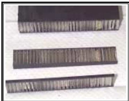
Figure 2: Illustration of the as-cut specimen after sectioning using the Model 850. The cut edges are very clean and exhibit no damage to the microstructure contained in the composite material. Cutting times were on the order of 10-15 minutes.
