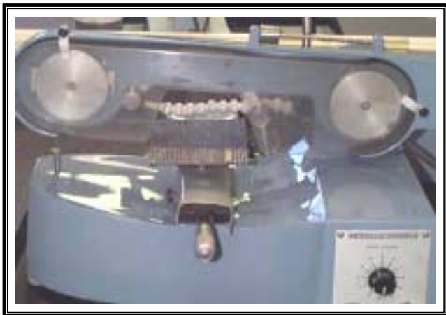
Figure 1: Image showing the composite sample as mounted onto the Model 850 Wire Saw. The sample is placed between the two larger pulleys and the sample is aligned to the wire blade. Sections are cut consecutively and the sample is advanced using the micrometer controlled stage.
