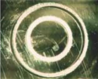
**Figure 2:** OLM image of the as cut surface of GaAs following the cutting procedure. The outer diameter of the specimen was cut first, with the inner diameter cut following the first cut. The inner cut is only about 1/3 of the total thickness of the specimen which will be used for planarity measurements following the cutting procedure.
