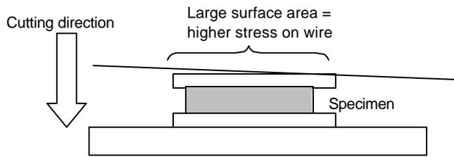
Figure 2: Illustration of the cutting process, showing the effect of surface area on the wire. In this configuration the wire is in constant contact with a large surface area of metal, causing stress and friction between the two, ultimately leading to wire failure.
