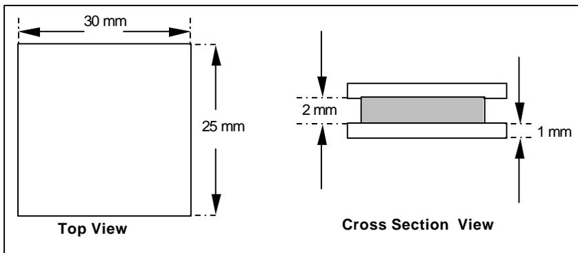
Figure 1: Schematic illustration of the specimens to be sectioned. The primary interest is the interface between the adhesive (gray area) and the stainless steel plates. Wire sawing will be used to preserve the interface region during cutting and to reduce any lapping and polishing steps to a minimum.
