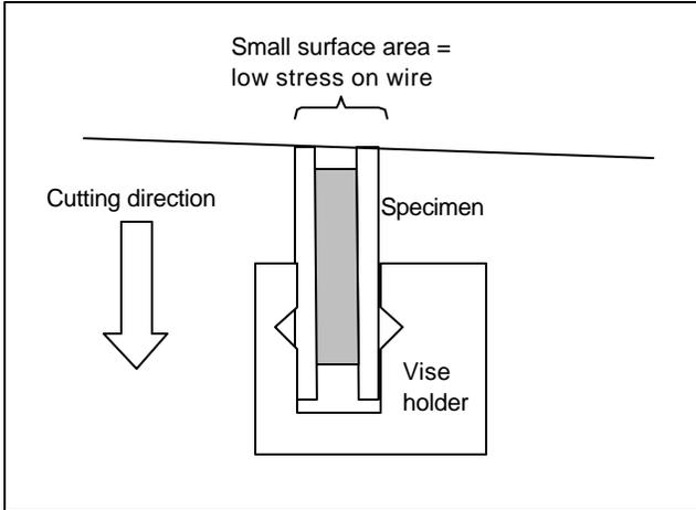
Figure 3: Illustration of the more efficient method for cutting these composite materials. By orienting the specimen vertically, the smallest possible cross sectional area was presented to the wire blade, which in turn reduced the friction on the wire and allowed sectioning of the device with precision. This method also produces straighter cuts due to increased support on both sides of the wire blade during cutting.
