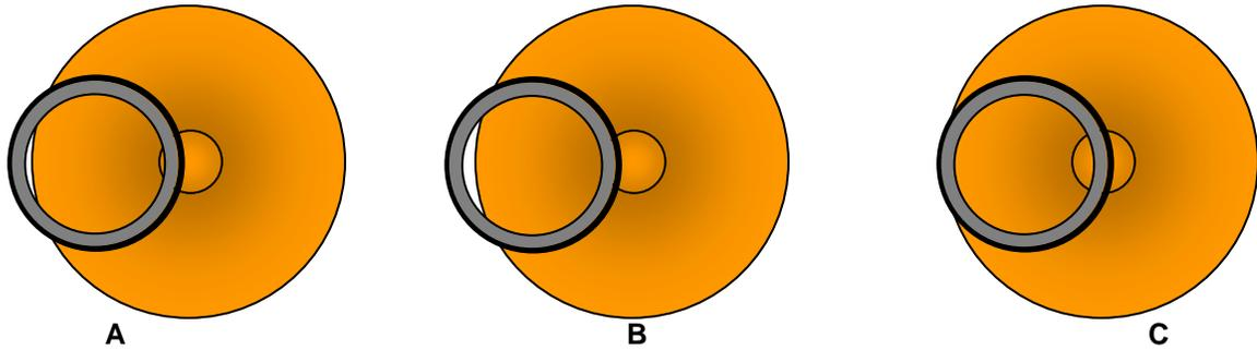
**Figure 2:** Schematic illustration of the conditioning ring positions during plate conditioning.
