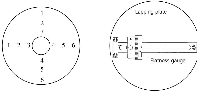
**Figure 4:** Schematic illustration of the locations used for measuring plate flatness (far left) and the orientation of the flatness gauge on the lapping plate during measurements.
