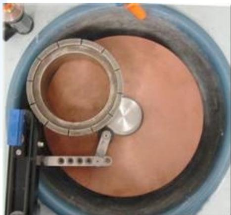
**Figure 1:** Image showing the Model 92002 Workstation with a diamond-conditioning ring. The ring is used for removing material from the lapping plate surface to create a flat surface for lapping processes.
