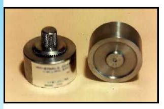
The Graduated Grinding Jig is used for grinding discs to accurate, predetermined, thicknesses prior to electropolishing.
