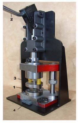
Precision engineered press for TEM discs
