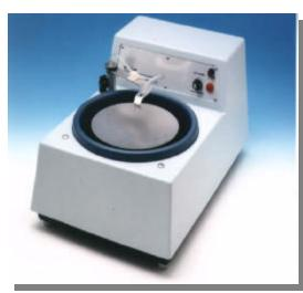
The Model 910 is the first in a new generation of multi-purpose lapping machines designed for accurately lapping and polishing a wide range of materials. The 910 can be used as a standard metallurgical grinder/polisher utilizing abrasive papers, abrasive films, diamond discs, polishing cloths, etc. Or it can be used as a high precision free abrasive lapping machine for flat polishing of optical and semiconductor materials.
