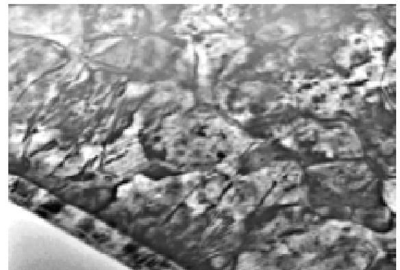
Wedge polished sample of tungsten over Ti-nitride/silicide over silicon at the edge of an oxide filled trench. (Image courtesy of IBM Analytical Services)
