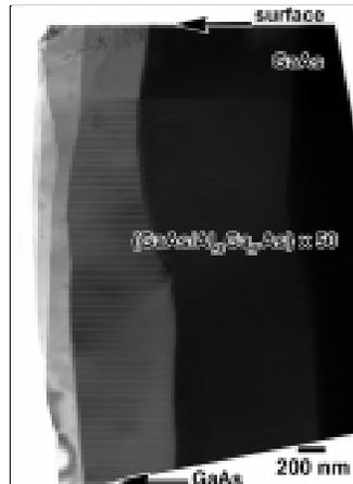
A Multiple Quantum Well structure grown by MBE showing the thickness terraces possible with a *MicroCleave™* sample. Image Courtesy of Scott Walck - Materials Directorate WPAFB. (Now with PPG Industries)
