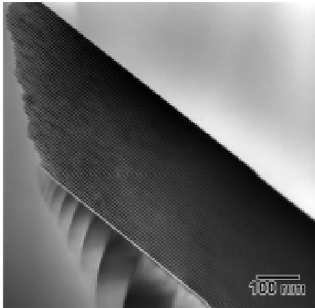
An X-ray mirror consisting of 45 layers of alternating Mo/amorphous Si (7.0nm period) on a Si substrate. Image courtesy of John McCaffrey - National Research Council of Canada.
