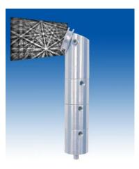
Pre-Tilt EBSD specimen stage with multiple height adjustment segments. Samples are kept at fixed 70° or 20° for EBSD analysis. The stage can be stored with a specimen in the SampleSaver<sup>TM</sup> storage container.
