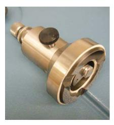
Two SEM pin mount stubs can be mounted into a modified specimen mount to fit an SBT model 150 micrometer controlled lapping fixture for polishing. The specimen remains attached to the stub during polishing and can be transfered directly to the SEM or stored and transported in the SampleSaver™ storage container.
